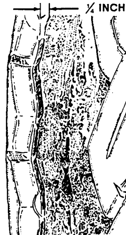
INSUFFICIENT AMOUNT OF UNDERTREAD
